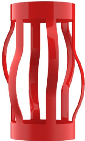
Designed with a precisely formed cross bow curvature, the UROS-CT has no 'knife edges' to reduce the risk of subsea well head damage on insertion. This also adds additional strength to the bows.
