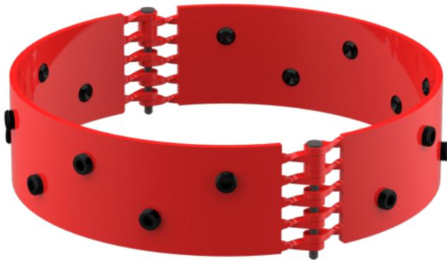
Each HDSH stop collar is made from the same patented steel as our heavy duty S2-HD centralizers. Like the S2-HD these stop collars are heat treated for strength and tempered for resilience. This ensures that the HDSH can withstand high axial forces, making it suitable for demanding well conditions.
