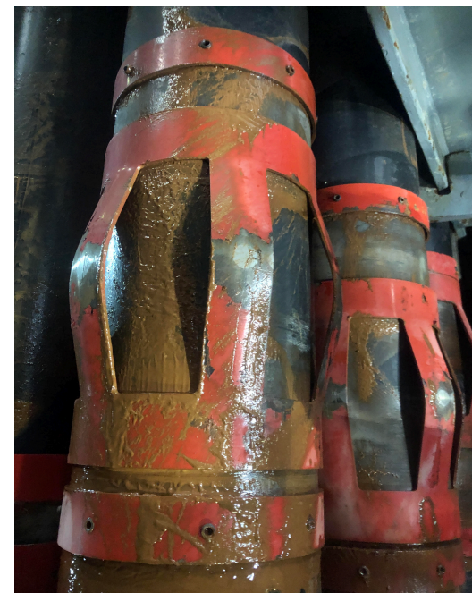
Undamaged centralizers after being POOH
