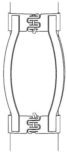
Bend hinge pins to secure centralizer onto casing
