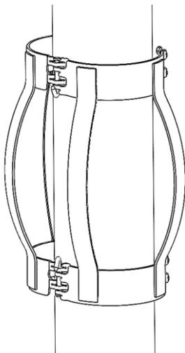
Hinge centralizer assembly onto casing
