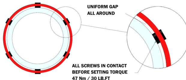
**Apply torque @ 30 lb.ft. (40.7Nm)**
