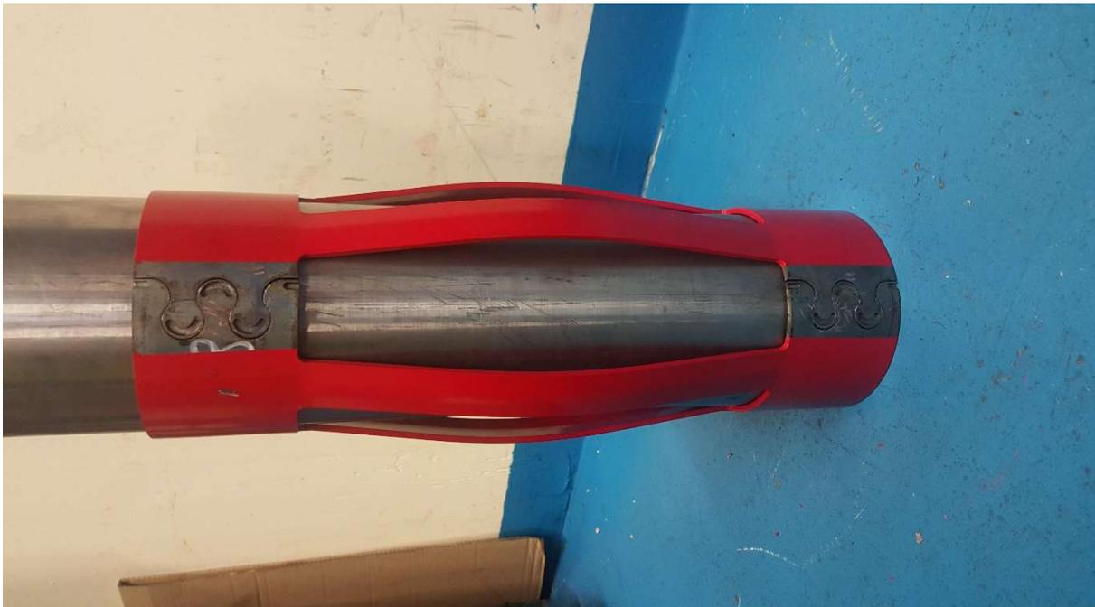
7. At this point the weld procedure can be followed in order to weld the centraliser interlocks together.
