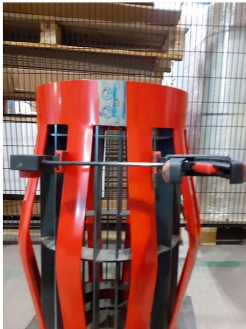
9. If the interlock gap exceeds 1mm when fitted to the pipe (pre-weld), then use a clamp on the bows to gently pull the interlock gap together.
