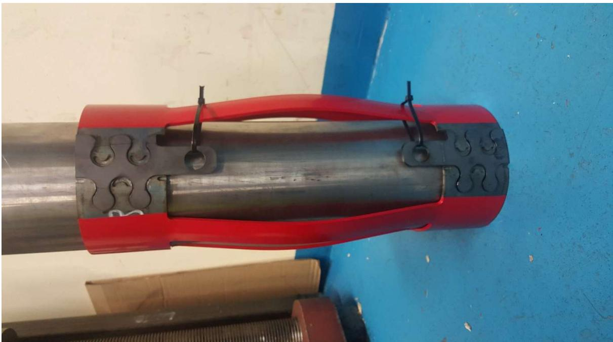
5. Once in place, use a mallet to hit directly downwards on the centraliser at the side of the interlock, this will allow the interlock spacers to spring clear of the centraliser, but will be retained from causing injury by the cable ties.
