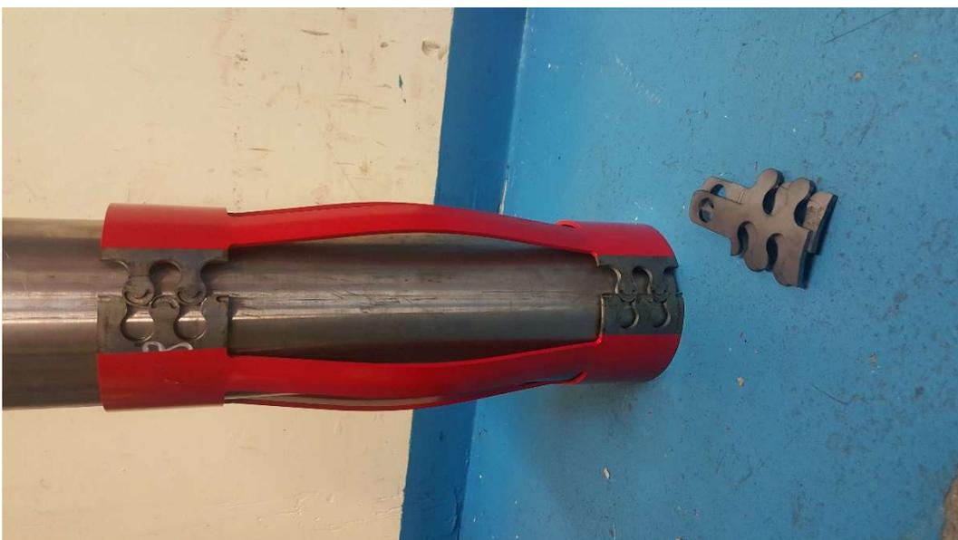
7. To interlock the centraliser fully hit downwards again on one side of the interlock and this will persuade the segments together.
