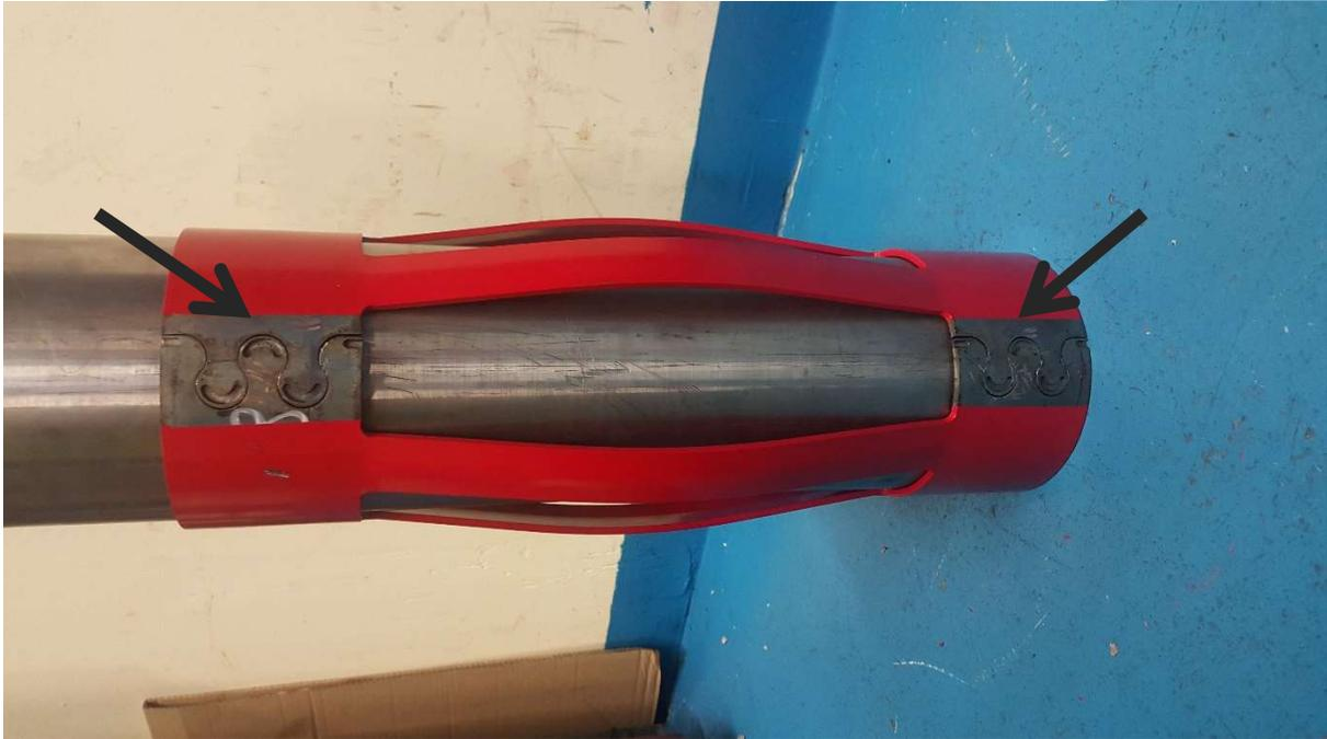
8. At this point the weld procedure can be followed in order to weld the centraliser interlocks together.
